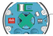
büS service interface Connection for CAN adapter or USB-büS interface set
